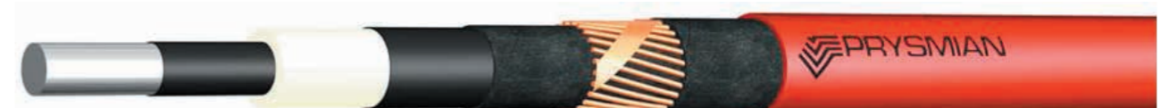
Delft MV 1-core cable with solid aluminium conductor, XLPE or P-laser insulation, copper wire screen and PE outer sheath
