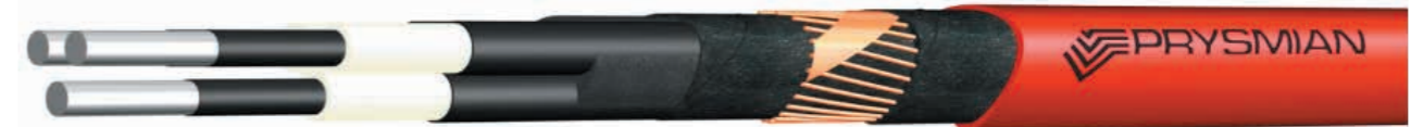
Delft MV 3-core cable with solid aluminium conductors, XLPE or P-laser insulation, copper wire screen and PE outer sheath
